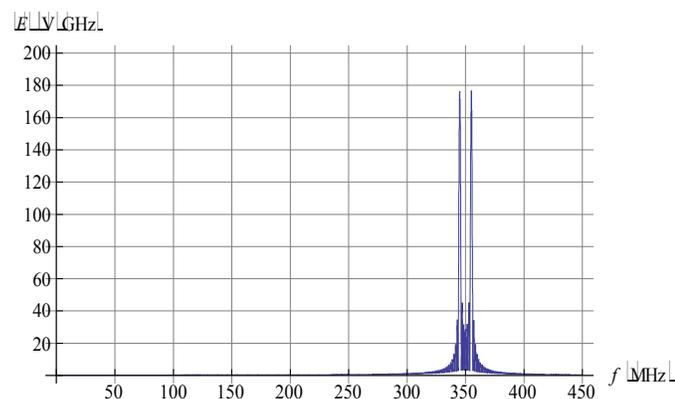
Fig. 7. Amplitude spectrum of the electromotive force shown in Fig. 6.
