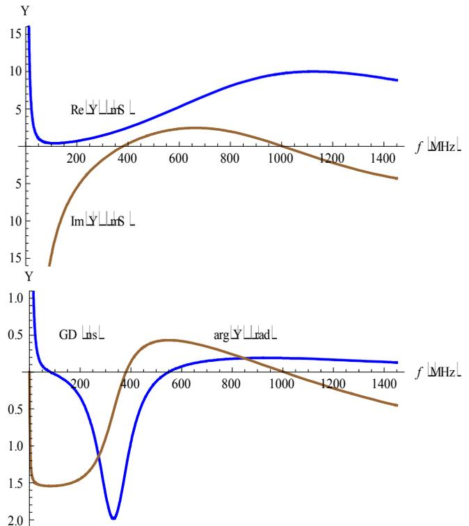
Fig. 5. Real and imaginary parts, group delay, and argument of the input admittance of the network shown in Fig. 4.
