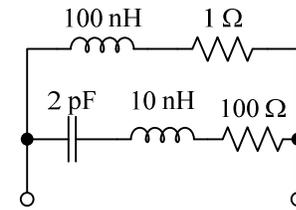
Fig. 4. Lumped-element equivalent network of a coil.
