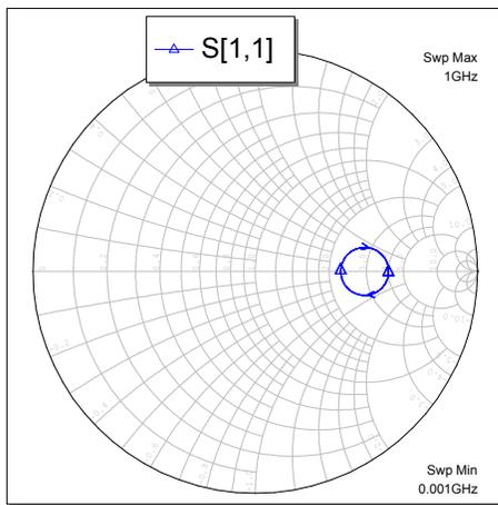
Fig. 2. Input reflection coefficient of the network shown in Fig. 1.
