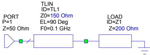
Fig. 1. A transmission line mismatched at both ends.
