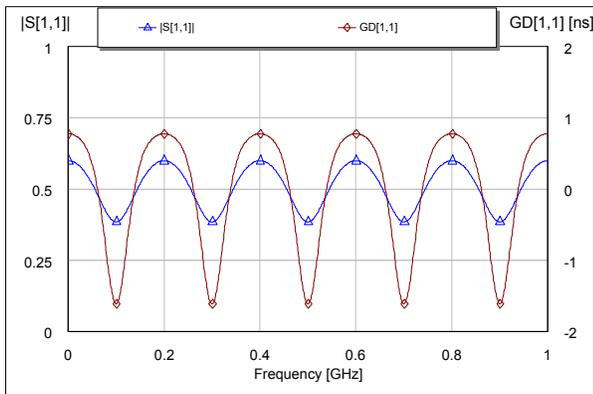
Fig. 3. Modulus of the input reflection coefficient and the group delay of the network shown in Fig. 1.
